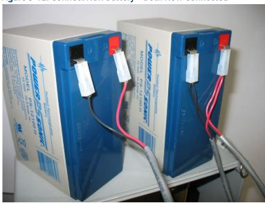
Figure 5-12. Connect New Battery – Both Now Connected
