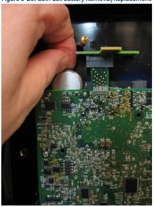
Figure 5-20. Coin Cell Battery Removal/Replacement
