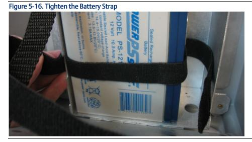
16. The strap includes a narrow opening into which you can slide the other end of the strap to help you tighten it.
