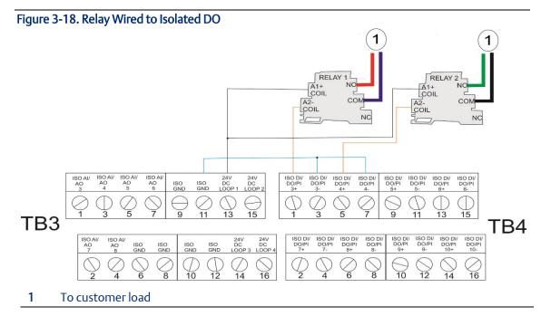
Alternatively, you can wire a relay to a non-isolated DO (*Figure 3-19*). In that case, you must use the non-isolated GND and provide 24V to power the relay. To attach a wire, insert it into the connector and tighten the adjacent screw to secure it. The NO and COM wires go to your external circuit or device.
