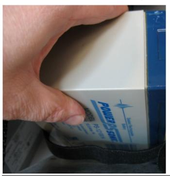
Figure 5-15. Ease the Battery into the Battery Compartment
