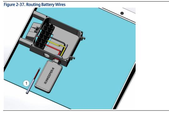
7. Connect the wires as shown. Replace the junction box cover.
