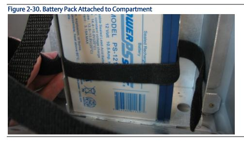
**5.** The strap includes a narrow opening into which you can slide the other end of the strap to help you tighten it.
