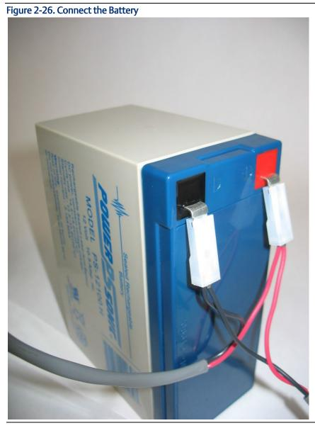
6. Now you must secure the battery in the battery compartment so that it doesn't move around. How you do this depends on which battery compartment configuration you have. If the battery compartment includes a strap for holding the battery, see Section 2.10.2.1 – Securing the Battery with a Strap; if the battery compartment includes an adhesive pad, see Section 2.10.2.2 – Securing the Battery to the Pad.
