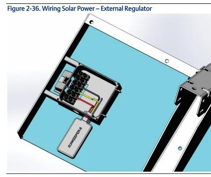
6. Route the BATT+ and BATT– wires from the flow computer into the junction box.
