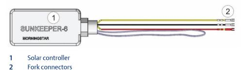
3. Remove the fork connectors and trim back the insulation on the wires 1/4 inch.
