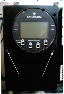
Figure 5-19. Remove the CPU Enclosure Cover
