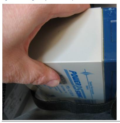
Figure 2-29. Easing Battery Pack into Compartment
